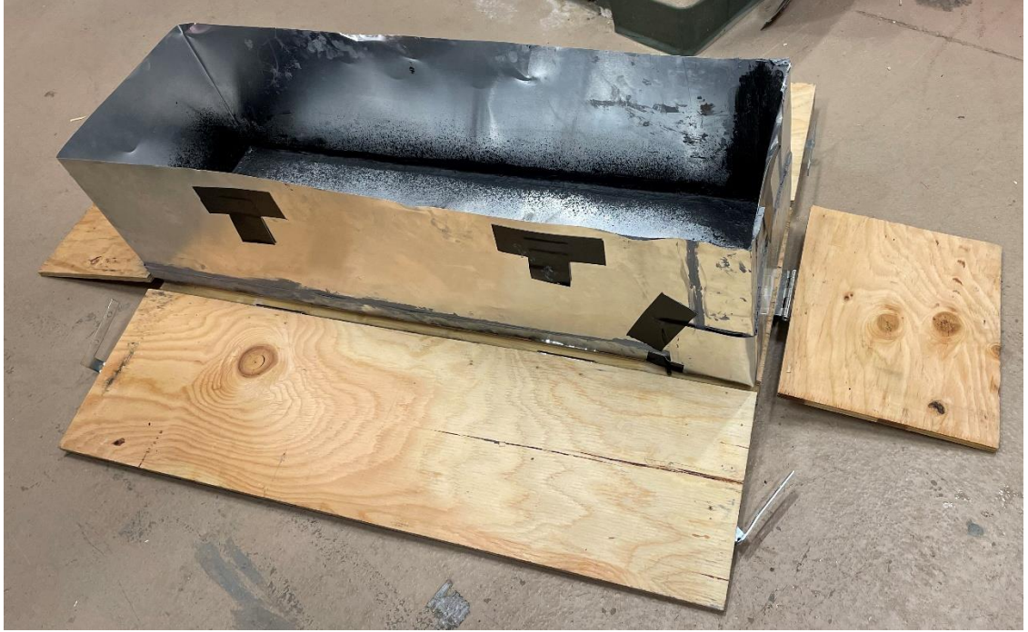
Figure 27: Wooden box for ice block with sides collapsed.
