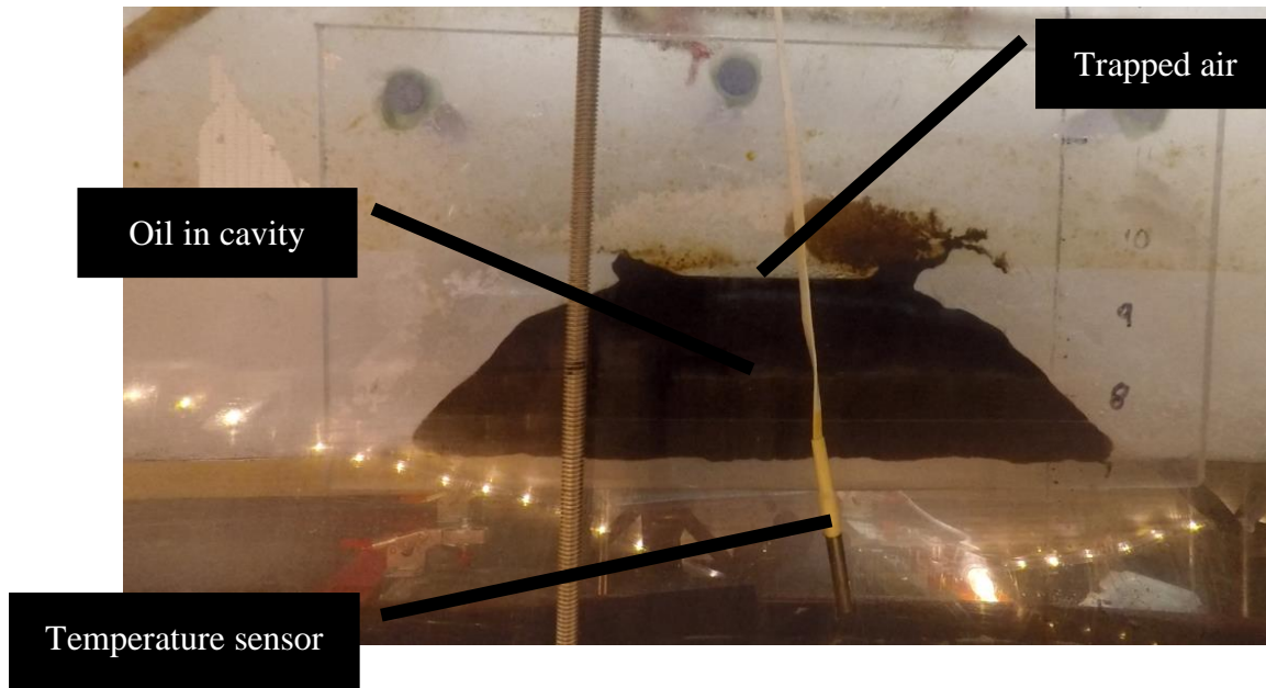
Figure 57: Side view of oil and air in cavity (3,054 mL oil injected) (run 1).
