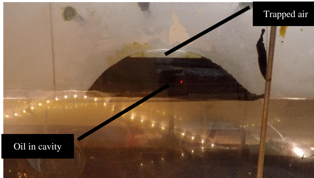
Figure 58: Side view of oil and air in cavity (3,022 mL oil injected) (run 2).
