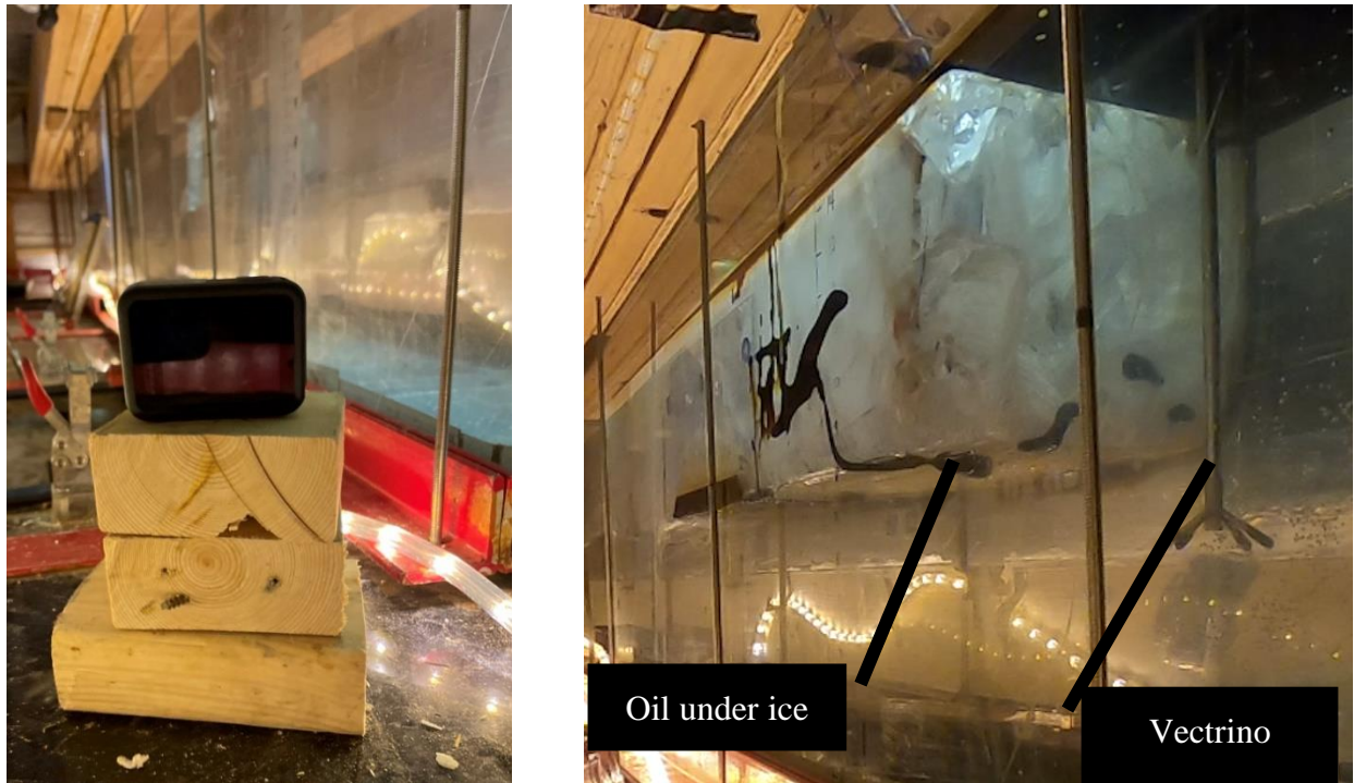
Figure 24: GoPro camera and its 3-dimensional view including downstream end of ice cavity and underside of ice.
