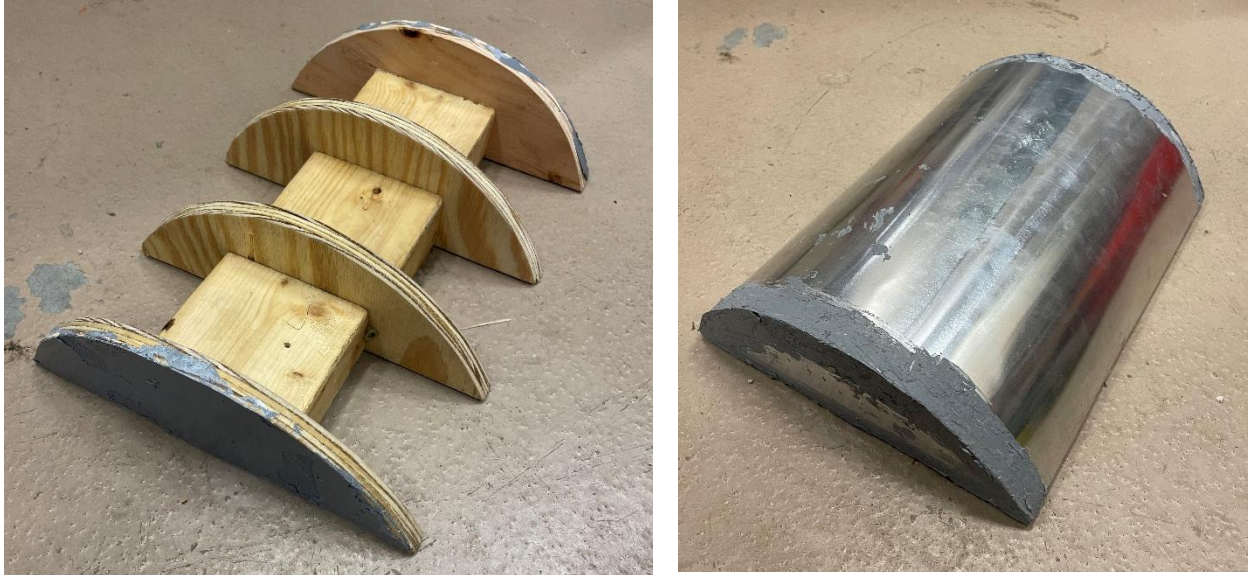
Figure 39: Mold constructed with wooden sections and sealed with aluminum flashing.
