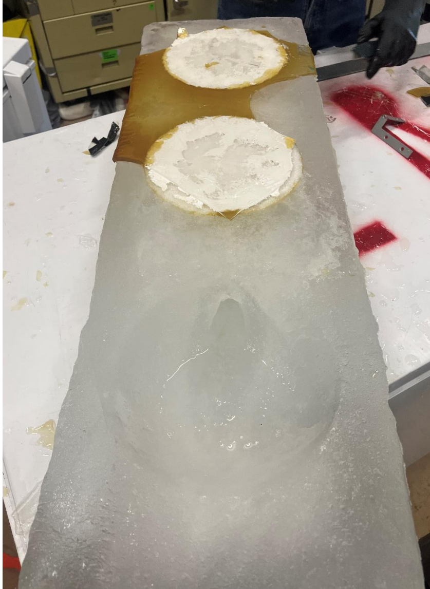
Figure 31: Fiberglass resin remained on bottom of ice block, as it snapped around molds (Styrofoam hemispheres).
