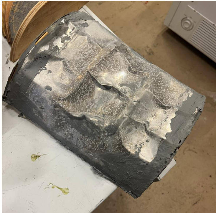
Figure 40: Attempt shaping mold from wooden pieces sealed with aluminum flashing and metal bond. Mold was not able to maintain its structural integrity from the pressure of the water freezing.
