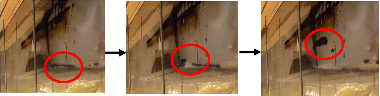
Figure 55: Ice melt evident due to oil pooling along bottom of ice and flowing laterally in path eroded in ice block.
