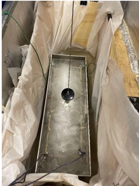
Figure 19: Warm water tank lined with plastic to loosen ice from welded box.
