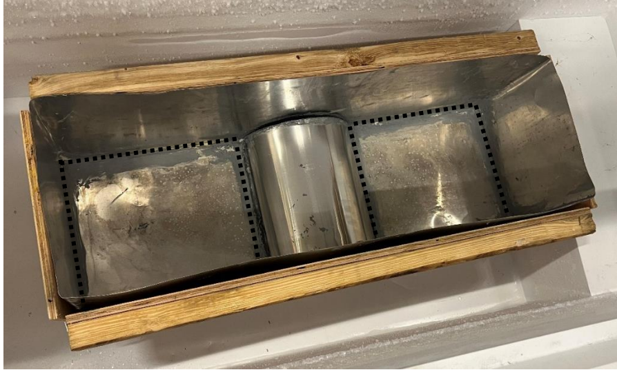
Figure 32: Attempt sealing aluminum flashing liner with metal bonding adhesive (dotted line), which was difficult to achieve and maintain a watertight seal. The liner was sealed along each bottom edge, along a side edge where the aluminum flashing overlapped, and along the edges of the mold.
