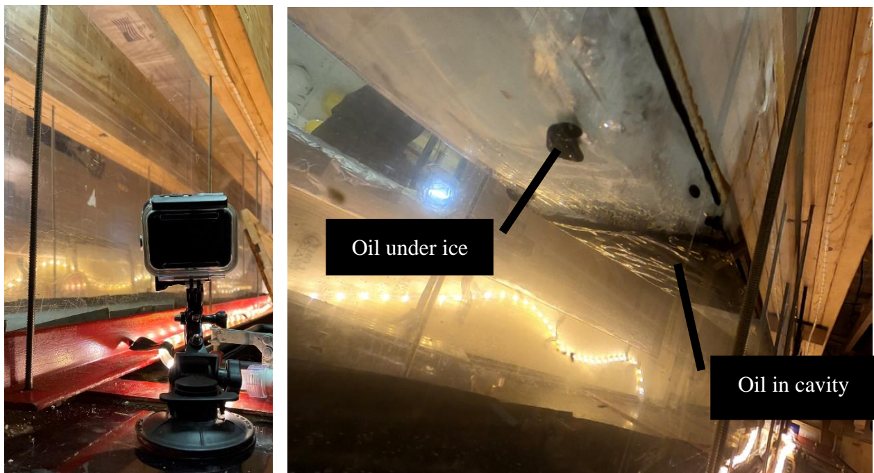
Figure 24: GoPro camera and its 3-dimensional view including downstream end of ice cavity and underside of ice.
