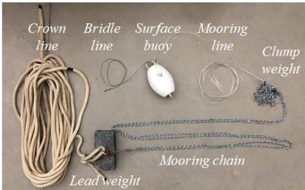
Fig. 4.9. Mooring components used for model tank testing.
