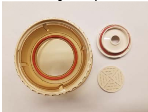
Figure 3. Proper gasket placement and dislodged filter plate.
