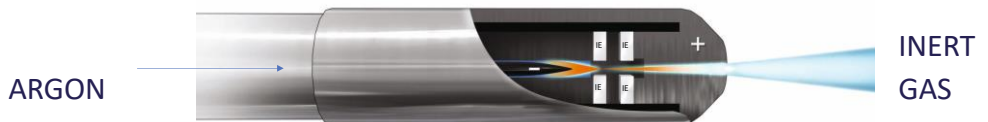
Figure 3 PlasmaJet device: argon gas is heated to generate plasma. (-) Cathode; (+) Anode; (IE) Intermediate Electrodes.
