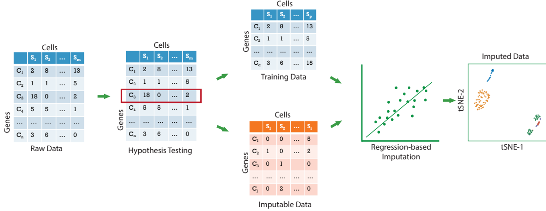
Figure 3.1: The overall pipeline of RIA. The algorithm consists of two modules. In the first module, we apply a hypothesis testing approach to determine which genes need to be imputed and which genes can be used as training. In the second module, we adopt the generalized linear model to impute the missing values from the imputable set. The algorithm outputs the imputed matrix that has the same number of rows and columns as of the input data.
