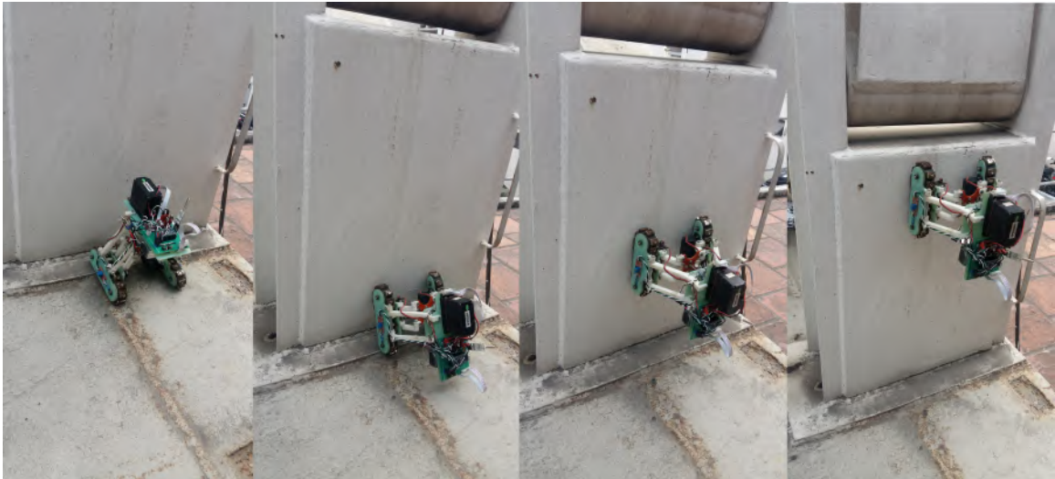
FIGURE 2.21: Adhesive and climbing test on a thick paint-coated steel structure: flat surface.
