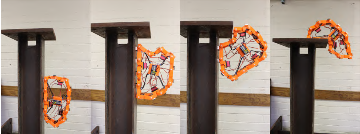
FIGURE 3.12: Robot test on an I-shape beam.
