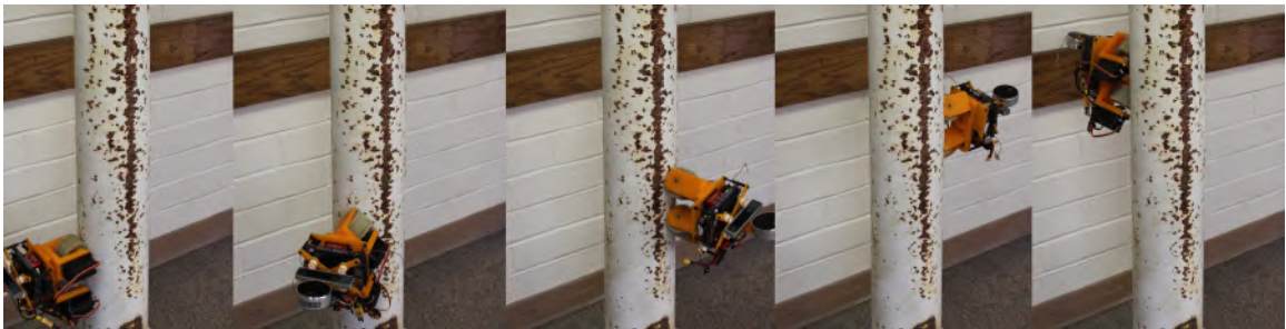
FIGURE 5.24: Thanks to free joint Figure. 5.3 makes the robot body flexible. Wheels fully adhere to any surface curvatures. Robot locomotion tests on a cylindrical structure.
