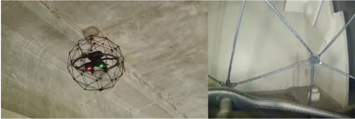
FIGURE 1.7: Elios 2, a commercial drone for visual inspection.
