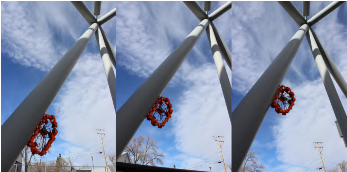
FIGURE 3.13: Robot test on a cylindrical beam.
