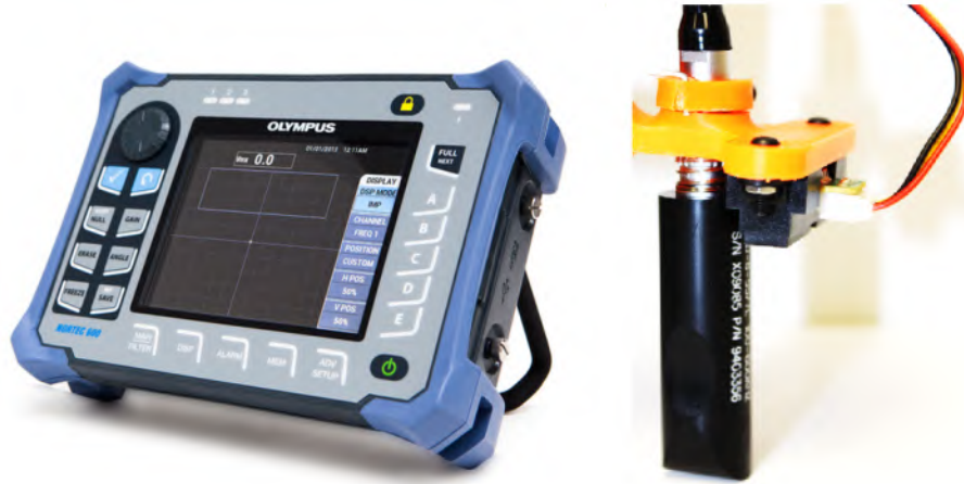
FIGURE 2.4: (Left) Industrial Eddy current sensor Nortec 600; (Right) sensor probe for data collection.
