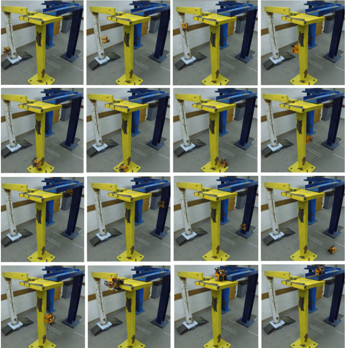
FIGURE 5.27: A complex structure setup for indoor experiments. It includes cylindrical, I-shape, U-shape, and rectangular steel frames. The robot can travel to almost any location except for discontinuous transitions and narrow spaces for robot size.
