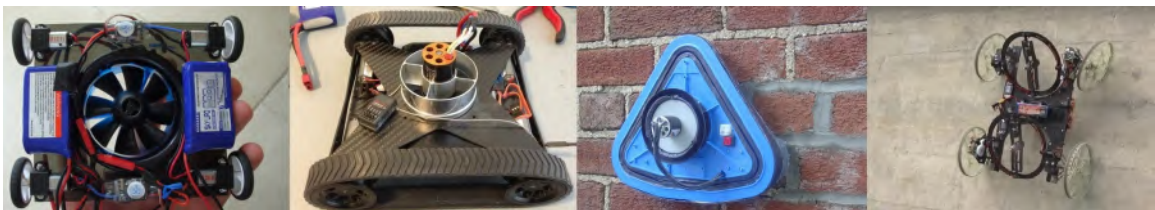
FIGURE 1.4: Robots utilize air pressure as an adhesive force to climb on structures.
