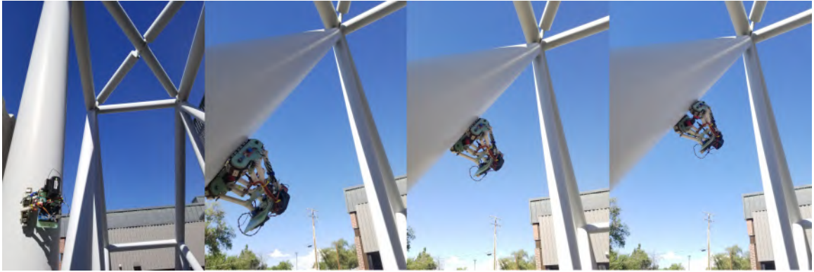
FIGURE 2.23: Adhesive and climbing test on a thin paint-coated steel structure: cylinder shapes D=250\text{mm} .
