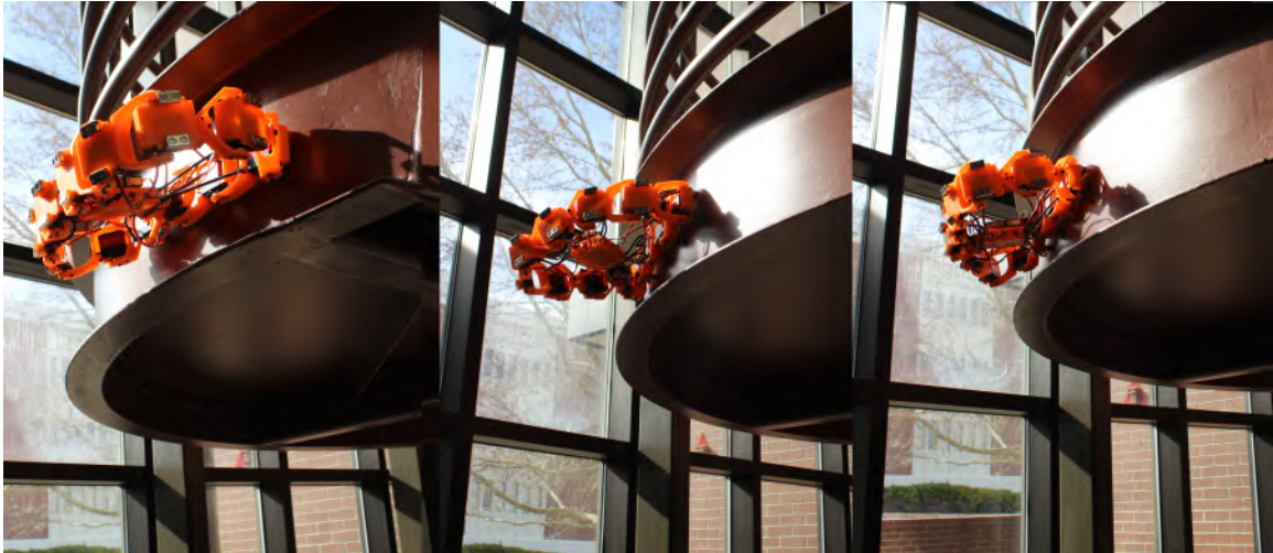
FIGURE 3.14: Robot test on a curved surface.
