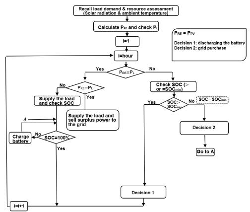
Figure 2. Optimization algorithm of grid-connected PV/battery hybrid energy system
