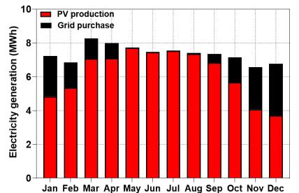
Figure 5. Energy generation profile of the optimal solution for cucumber-tomato greenhouse
