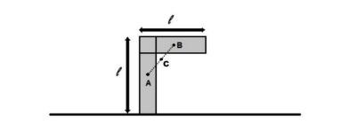
This object is going to topple over. And we might say that the object's toppling is caused by the center of mass being located outside of the base of the object. Gravitational force, G, pulls downwards at the center of mass which unbalances the normal force, N, at the base of the object (Shankar, 2019, pp. 119–127).
