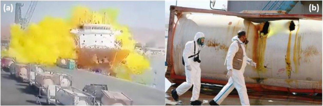
Figure 2- (a) Frame capture of the Aqaba Port incident, taken seconds after the chlorine tank is accidentally dropped (Akour, 2022). (b) Forensic experts evaluate the tank after the accident (Photo by Mazraawi, 2022).
