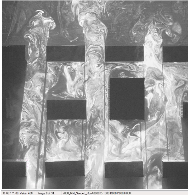
Figure 45 - Top view of a simulation of a chlorine release in the model with seed particles, used to determine the time interval between release and arrival at the channels in the last rows of the MUE.
