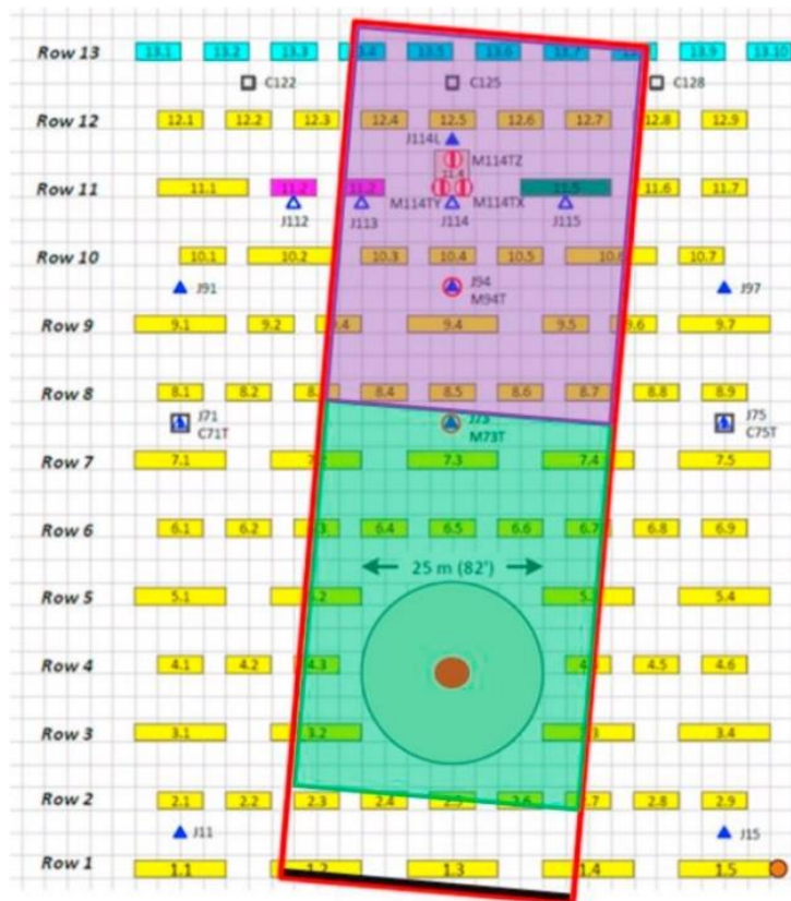
Figure 16 - Overlap of the MUE layout from JR-II to the water tunnel used by Owkes and peers. Concentration measurements were made in the green zone, while velocity measurements were taken in the green and pink zones (Owkes et al. , 2020).
