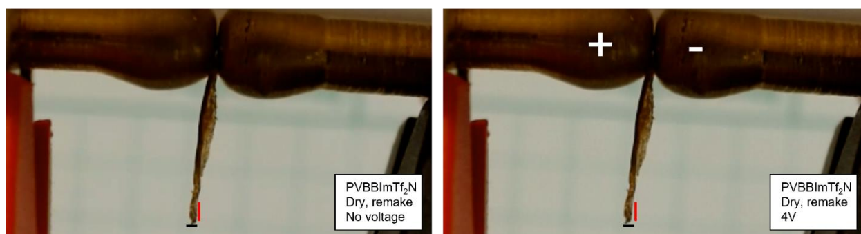
Figure E.21 PVBBImTf 2 N dry replicate actuator video still frames (a) before voltage application and (b) after applying 4 V. The black and red lines mark the side and bottom of the actuator initial position to aid visualization of the actuator displacement.
