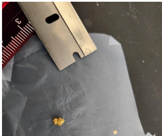
Figure E.19 PDMAEMA- b -PVBBImTf 2 N 25 wt% IL attempt at developing an actuator film with gold foil electrodes. After peeling from the Teflon sheeting, the film rolled up into a ball.
