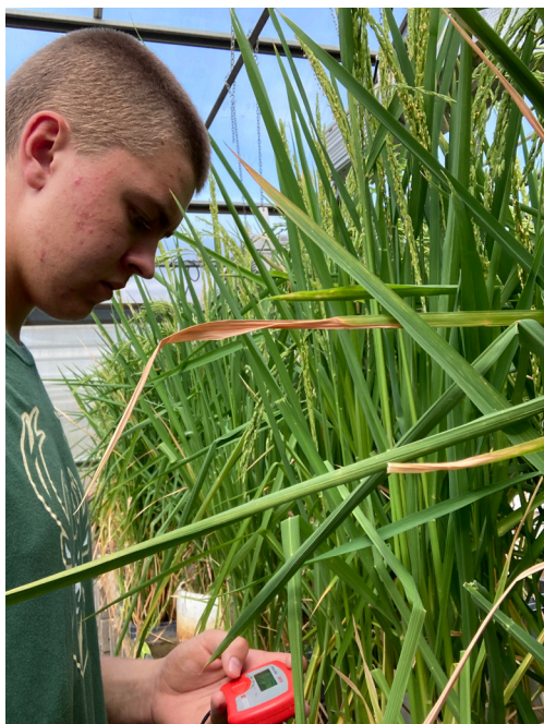
Jonathan Brye recording soil volumetric water content measurements within the furrow-irrigated-rice tubs in the greenhouse.
