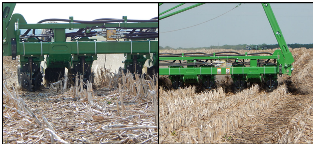
FIGURE 1 Soil displacement with the John Deere ExactEmerge 1775NT planter at 8 kph (left side) and at 16 kph (right side) planting speed in 2015.
