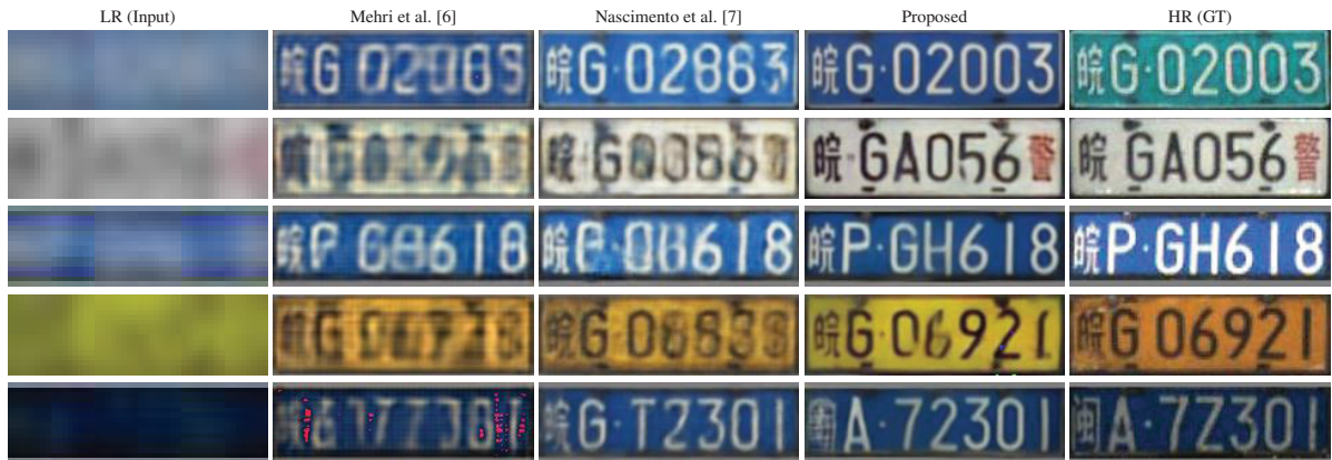
Figure 5.6: Representative examples of the images generated by the proposed approach and baselines in the PKU dataset [9].
