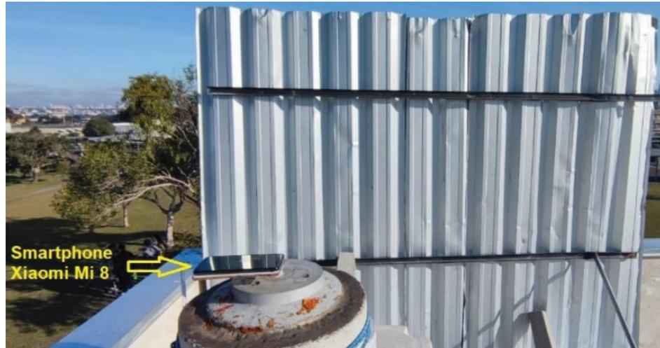
Fig. 5. Scenario 1: smartphone Xiaomi Mi 8 and the aluminum plate employed to generate multipath effect on GNSS signals.
