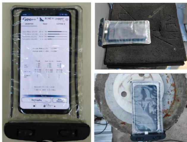
Fig. 7. Smartphone Mi 8 inside the water proof case.
