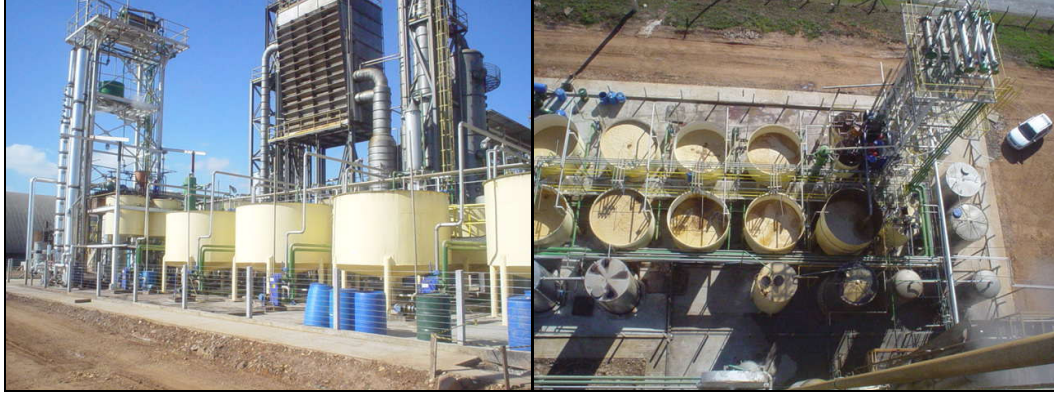
FIGURE 2 – INDUSTRIAL PLANT FOR ETHANOL PRODUCTION FROM SOYBEAN MOLASSES (10 m 3 ETHANOL PER DAY) SOURCE: Siqueira (2006)
