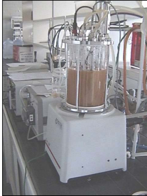
FIGURE 3 – INCELTECH BIOREACTOR SOURCE: Toro (2005)
