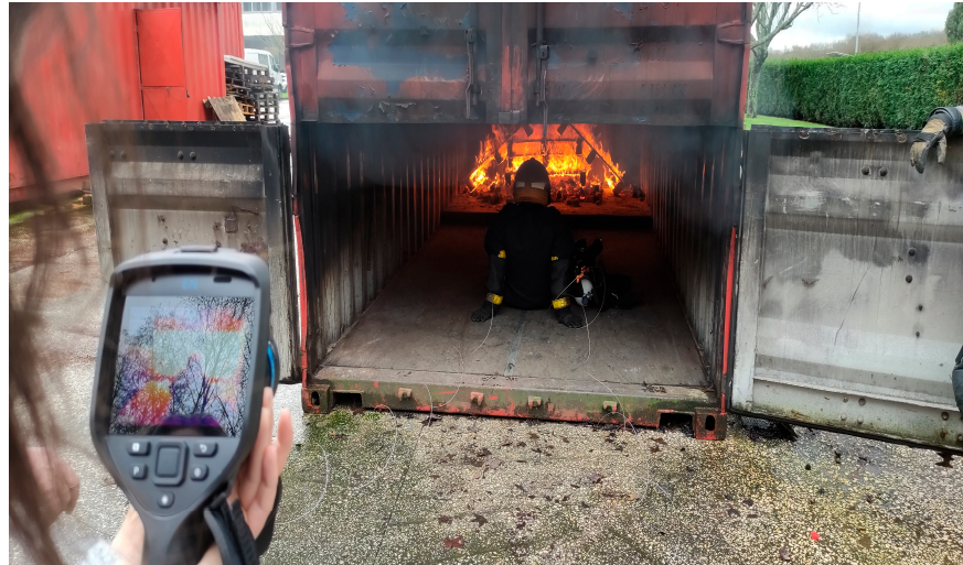
Figure 3. Simulated environment tests in the container used to simulate urban fire scenarios: temperature monitoring with a thermal camera.
