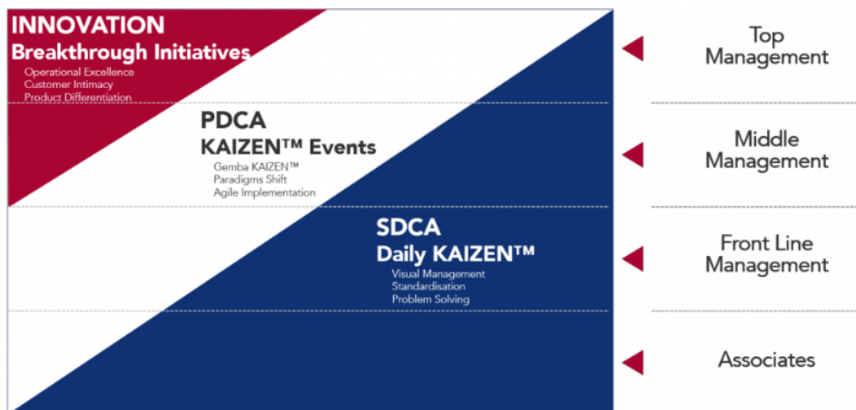
Figure 2.2: Kaizen Institute Flag. Innovation (red), Improving (white), and Standard Work (blue) are CI areas that leaders should implement according to their level in the organization. Source: Institute (2023a)
