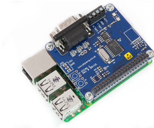
Figure 3.5: PiCAN2 shield for CAN interface mounted on top of a Raspberry
