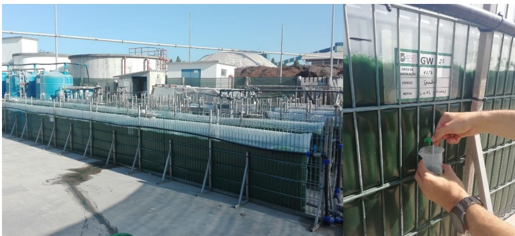
Figure 6. Cultivation of Arthrospira sp. in a flat panel photobioreactor with roughly 750 L in the medium MNS supplemented with NaHCO 3 at 16.8 g L -1 under outdoor conditions.
