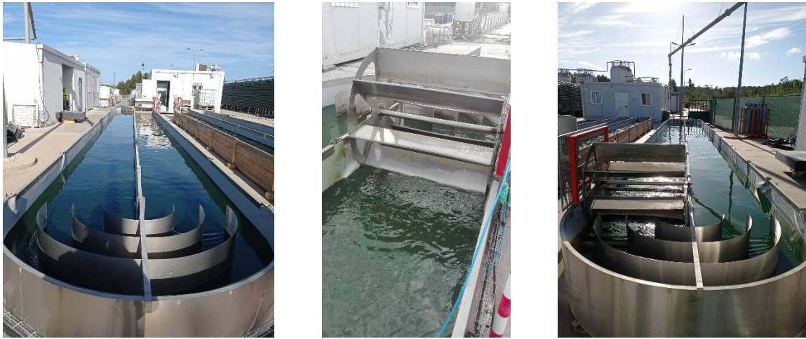
Figure 7. Cultivation of Arthrospira sp. in a raceway pond with a surface area of 27 m 2 and a working volume of 3.5 m 3 . Growth occurred in MNS with NaHCO 3 under outdoor conditions.
