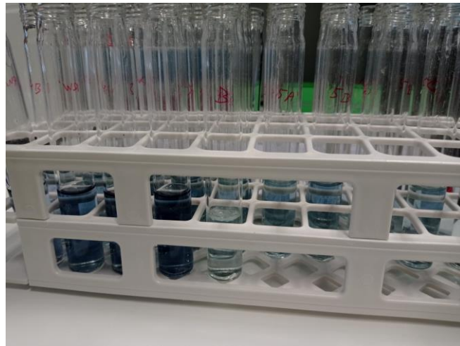
Figure 9. Glass tubes after realizing the extraction of protein from Arthrospira sp. by the Lowry et al. (1951) method.
