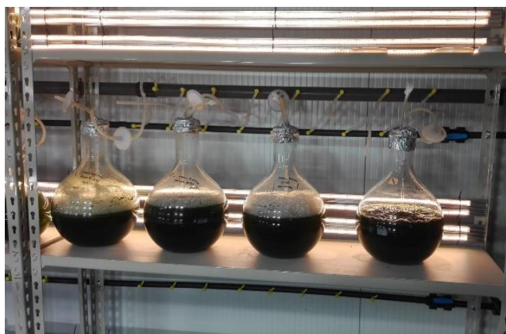
Figure 5. Arthrospira sp. growth in Zarrouk medium in 5 L reactors under laboratory-controlled conditions.
