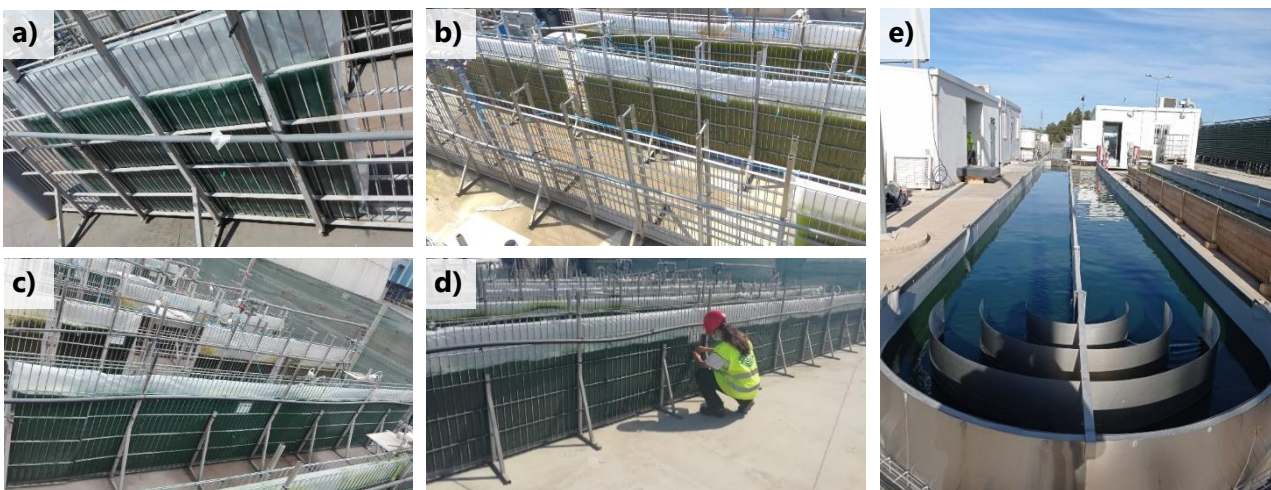
Figure 17. Reactors used in the scale-up of Arthrospira sp. (outdoors). (a) FPP 80 L, (Zarrouk); (b) FPP 150 L, (MNS+ \text{KHCO}_3 ); (c) FPP 500 L, (MNS+ \text{NaHCO}_3 ); (d) FPP 750 L, (MNS+ \text{NaHCO}_3 ) and (e) raceway pond 3500 L, (MNS+ \text{NaHCO}_3 ), where 2 assays were performed.
