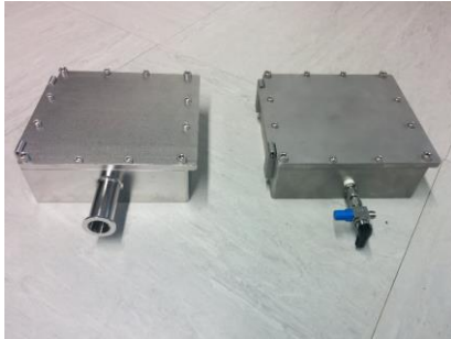
Figure 2.17. Photographs of helium leak test chambers and mass spectrometer.
