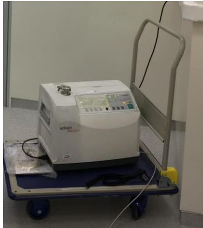
Figure 2.17. Photographs of helium leak test chambers and mass spectrometer.
