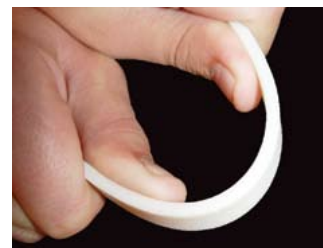
Accura® 25 Plastic has high flexibility, while retaining the original shape.
