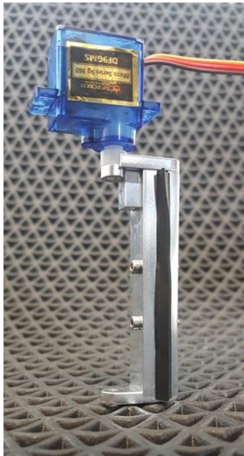
Figure 6.45 Wiper Support Parts and Servomotor
