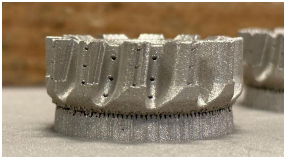
Figure 29 - Result of additively manufacturing the first iteration design
