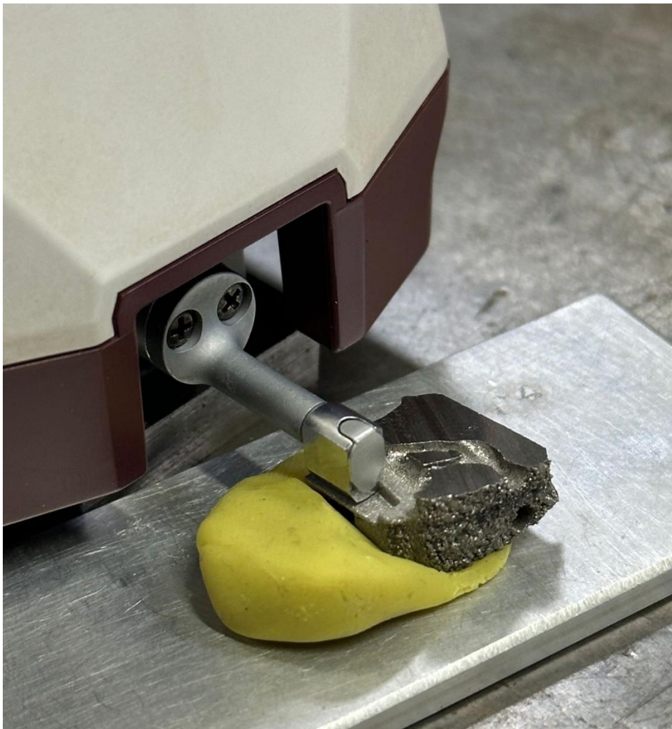
Figure 39 - Roughness measurement of the cutting edge
