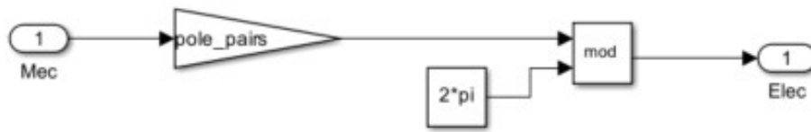
Figure 4.13: Angle Conversion Implementation
