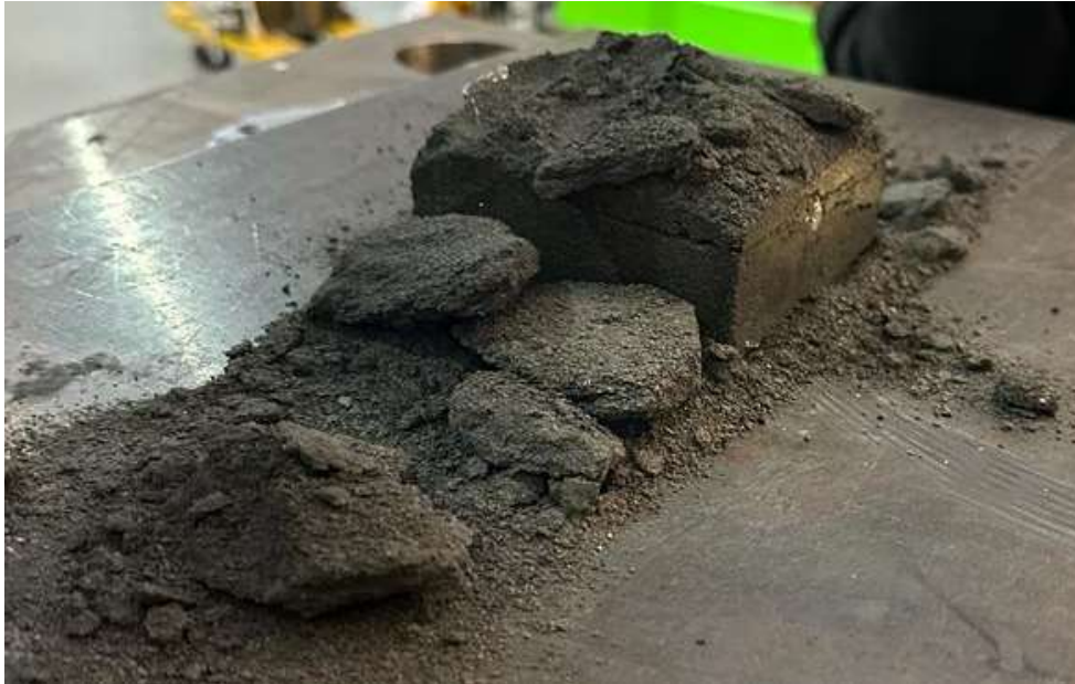
Figure 21 - Result after compacting of A356/Al 2 O 3 powder.
