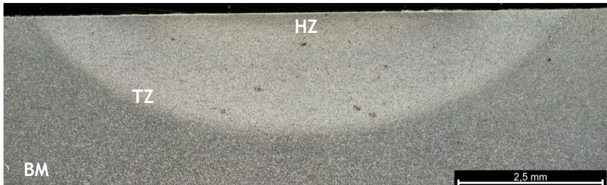
Figure 16- Cross-section of the laser surface hardened annealed base specimen with an interaction time of 16 seconds (A6) etched with a 2% Nital and 4% Picral mixture
