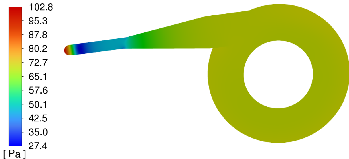
Figure 11 Contours of static pressure [Pa] inside the distribution ring for essay A.
