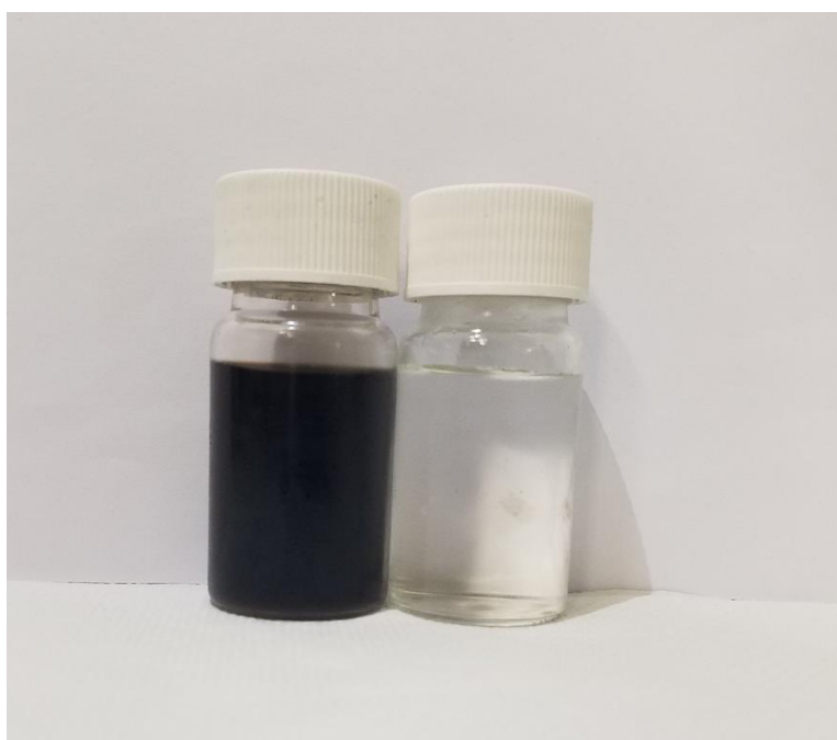
Fig. G.4. Color difference between the real effluent (on the left side) and the condensed phase of the same stream after the OMWSR process in the SEMR, at 400 °C and 4 bar (on the right side).
