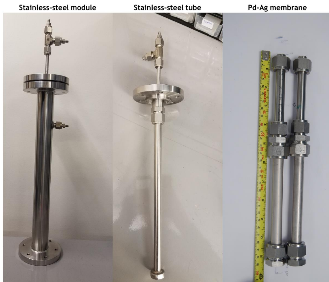
Fig. G.1. Module and tube/membrane used in the experimental tests.
