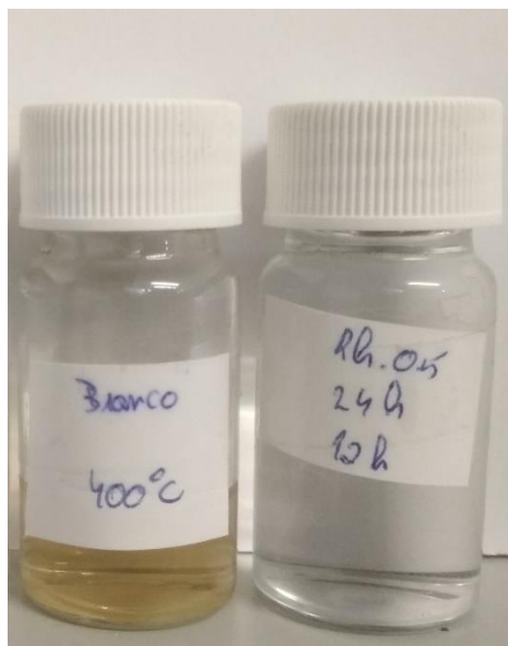
Fig. E.12. Color difference between the condensed phase obtained in the blank test (on the left side) and the condensed phase of the same stream after the OMWSR process in the stability test (on the right side).
