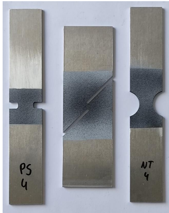
Figure 34 - AA6082-T4 calibration test specimens painted with a stochastic pattern.
