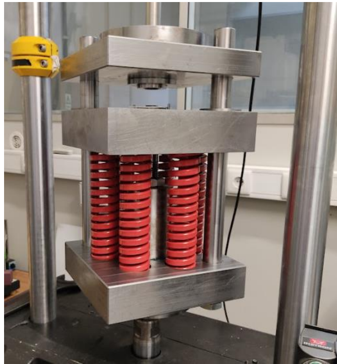
Figure 38 – Experimental equipment of the hole hemming process.
