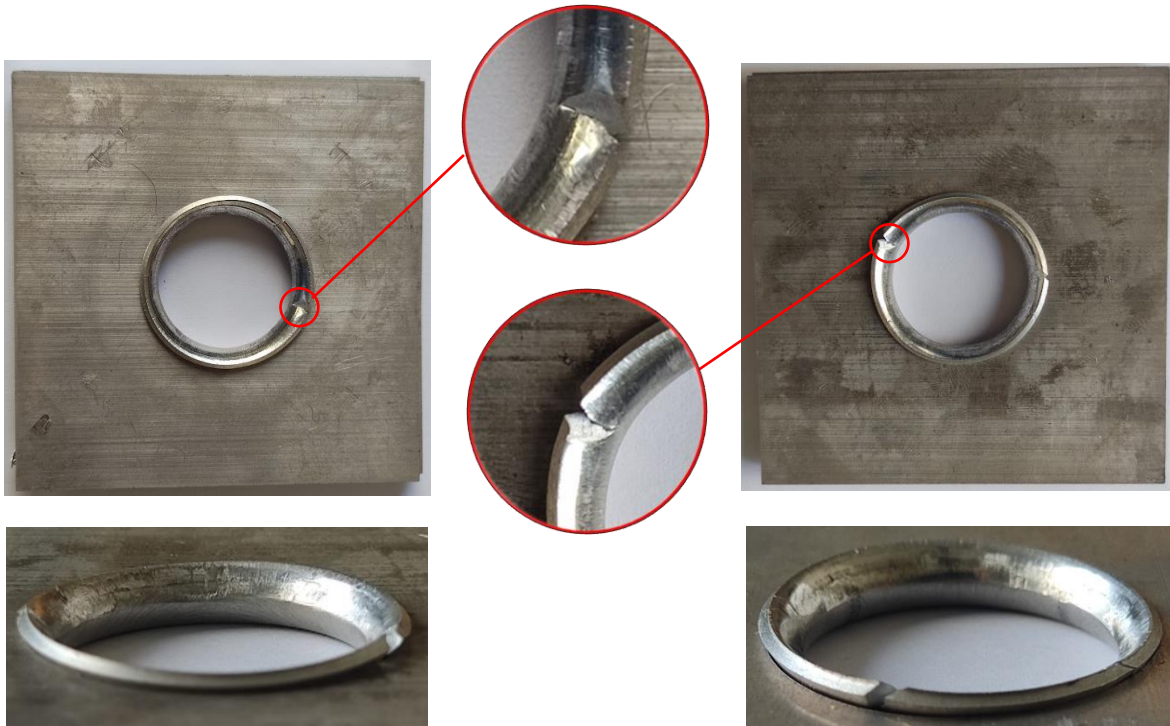
Figure 88 – Hole hemmed joints for the F = 4.5 mm case.
