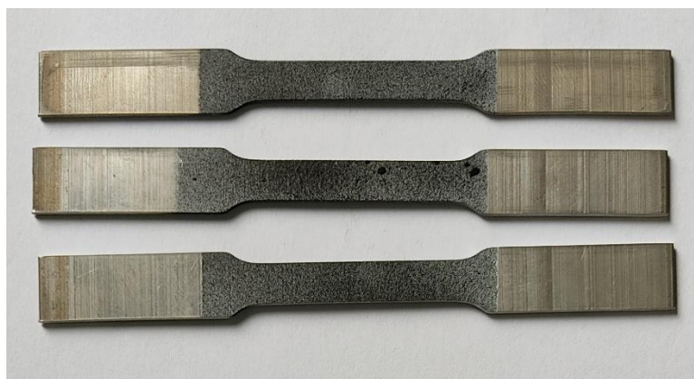
Figure 22 – AZ31 uniaxial tension specimens painted with a stochastic pattern.
