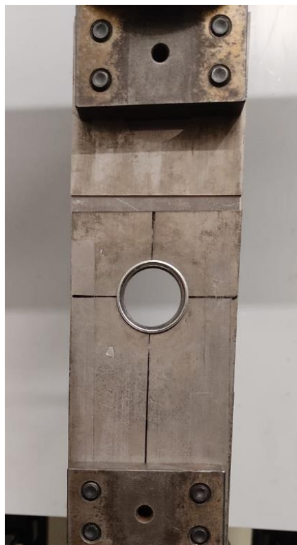
Figure 45 – Single lap shear test specimen fixed to the testing machine.
