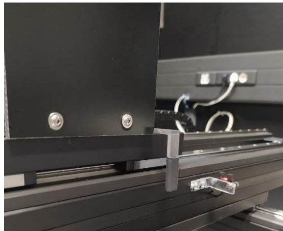
Figure 4.6 - Intermediate detector and its support parts of one of the horizontal axes
