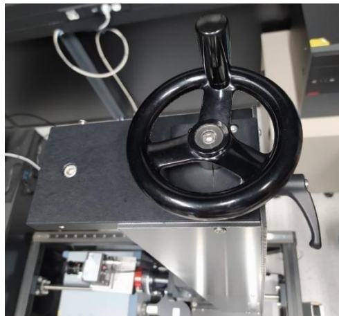
Figure 2.12 - Hand operated spring break with vertical hand crank
