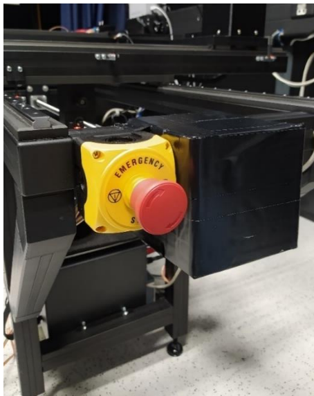
Figure 4.9 - Emergency button, protection part against gears and the protective box (below)
