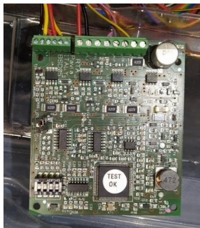
Figure 4.1 - BSD 02.V stepper driver
