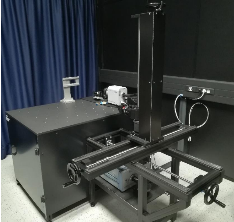
Figure 2.11 - Manual testing workbench with a LumiCan 1300
