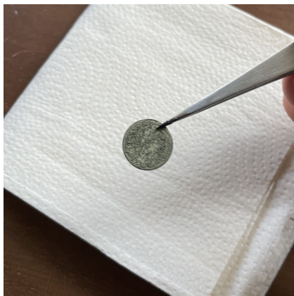
Figure 4.1: Cathode after being dried overnight in vacuum.
