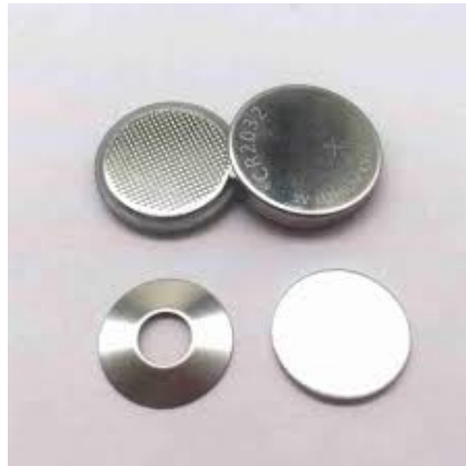
Figure 3.14: Components of a CR2032 coin cell [80].
