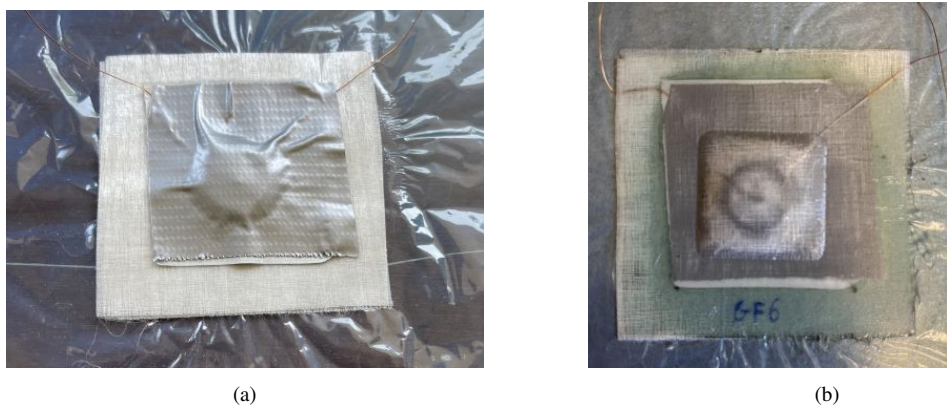
Figure 3.21: Duct tape as sealing agent (a) before and (b) after curing.
