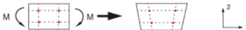
Figure 3.14: Linear fully integrated element behaviour under a pure bending load (the integration points are represented by the red dots) [Simulia, 2019].
