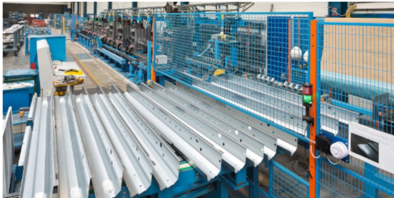
Figure 2.6: Example of punched profiles [Voestalpine, 2019b].
