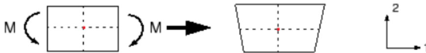
Figure 3.15: Linear element with reduced integration under a pure bending load (the integration points are represented by the red dots) [Simulia, 2019].
