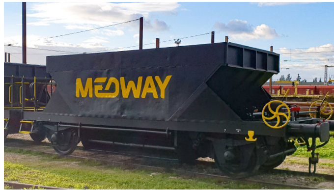
Figure 2.7: Heavy-duty Medway wagon for transporting ballast [32].
