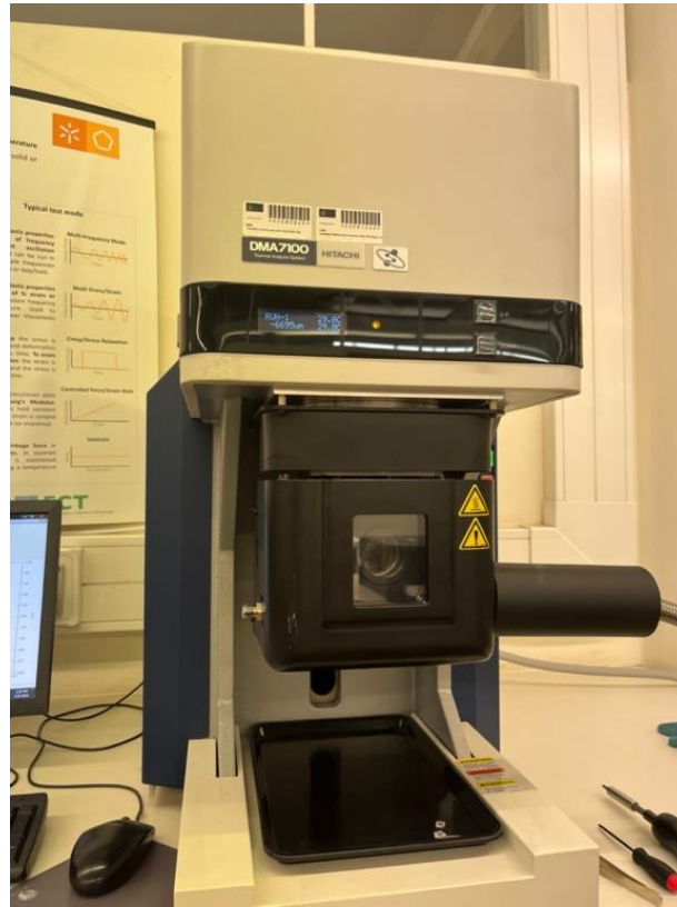
Figure 14: DMA7100 thermal analysis system used to determine the mechanical properties of porous-PDMS samples.
