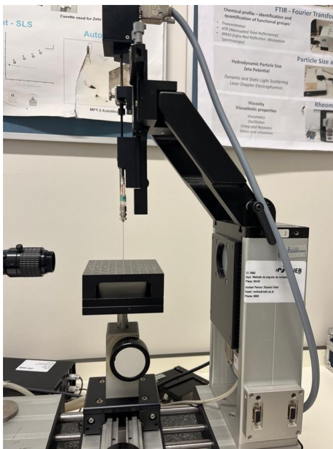
Figure 13: Dataphysics Instruments GmbH, Germany used to determine the wettability of the porous PDMS samples.
