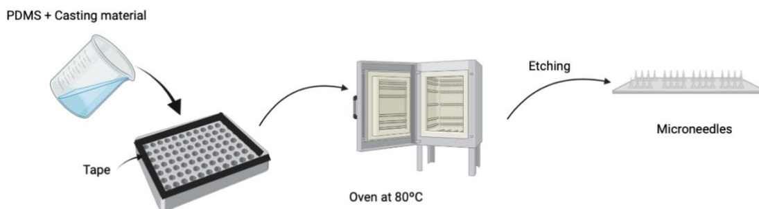
Figure 12: Schematic diagram representing the preparation of porous microneedle array.
