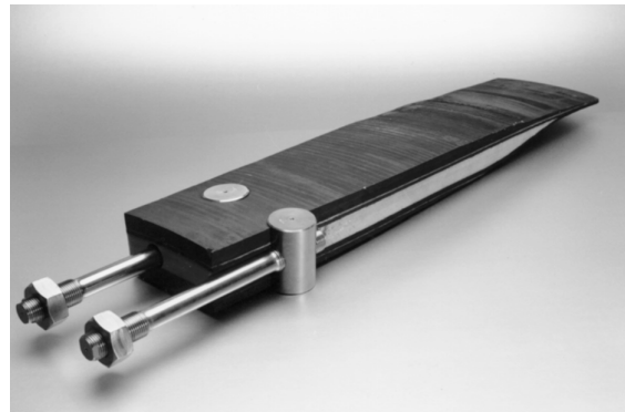
(b) Blade connection with cross-bolts [26]
