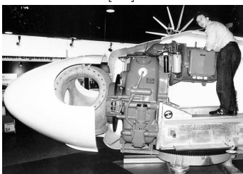
(c) Drive train of an earlier Nordex wind turbine, with rotor and generator attached directly to the gearbox [26]
