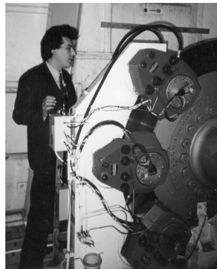
(b) Rotor parking brake at the low-speed side directly behind the hub in the earlier Howden HWP-1000 [26]
