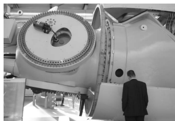
(d) Cast load-bearing structure with in-plane rotor bearing on a Vestas V90 [26]
