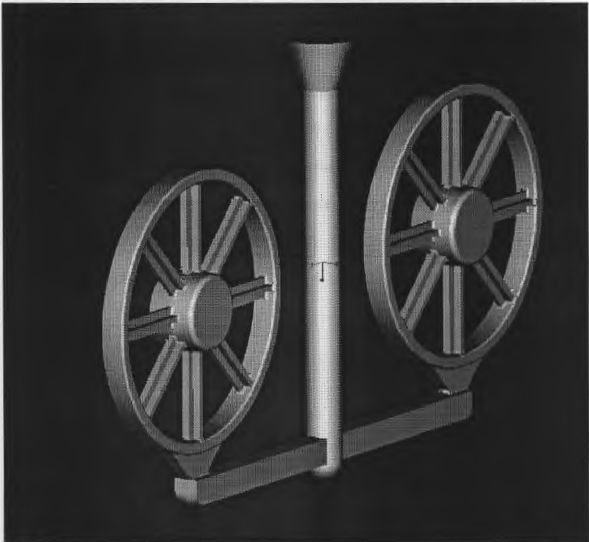
Figure 6. The vertical gating system design of permanent mold with two attached wheels.
