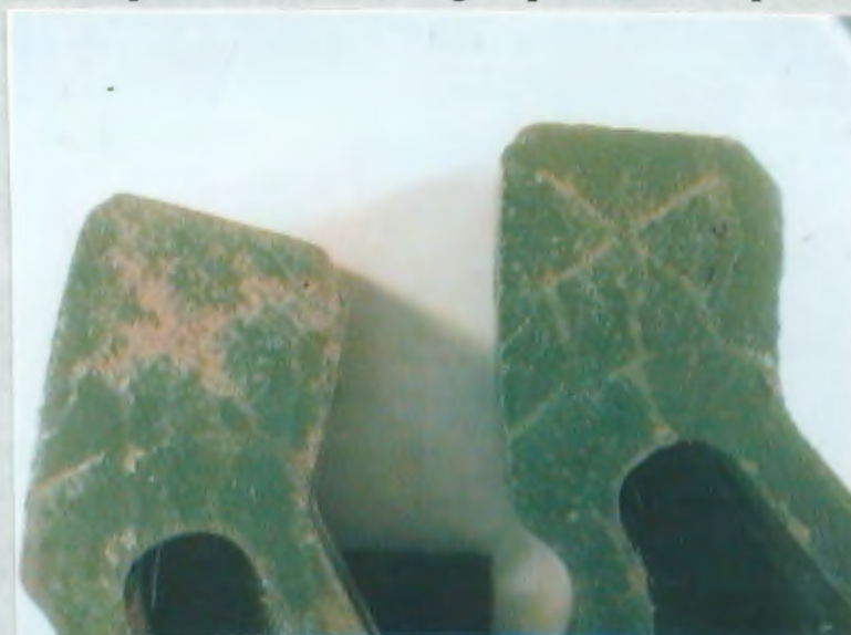
Figure 5: Salt Spray Test Creepback Examples Left panel baseline, Right panel autodeposition
