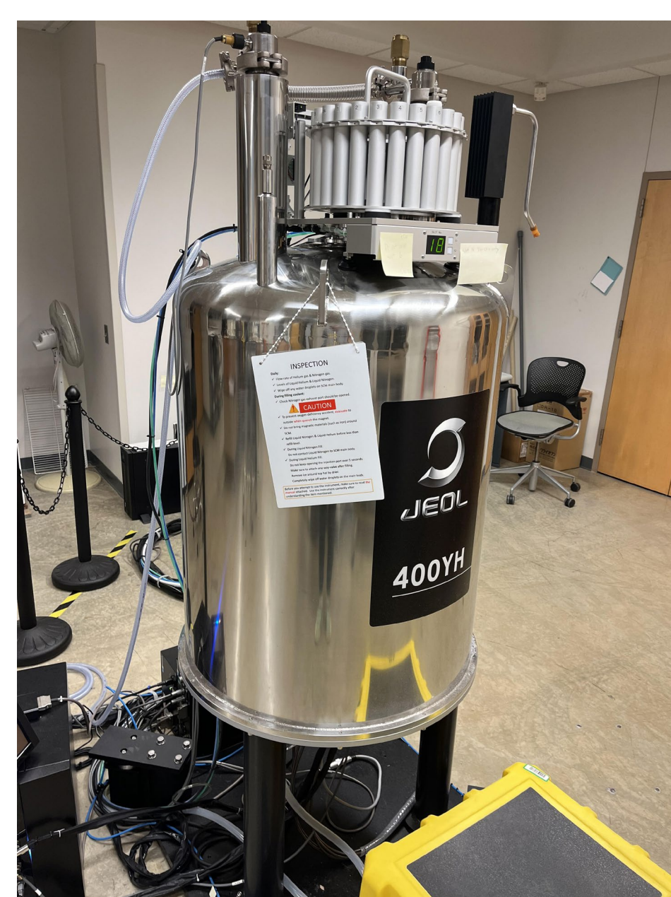
Figure 3. The nuclear magnetic resonance (NMR) spectrometer is how we are able to differentiate one compound from another by performing different tests with the spectrometer.
