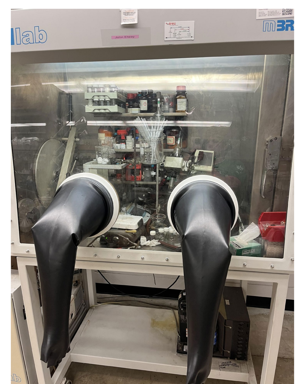
Figure 2. The dihydrogen complex is very reactive to air and moisture. The glovebox (above) is nitrogen filled giving the compounds an inert atmosphere.
