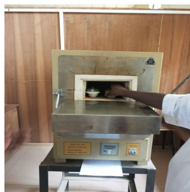
f) Muffle Furnace
