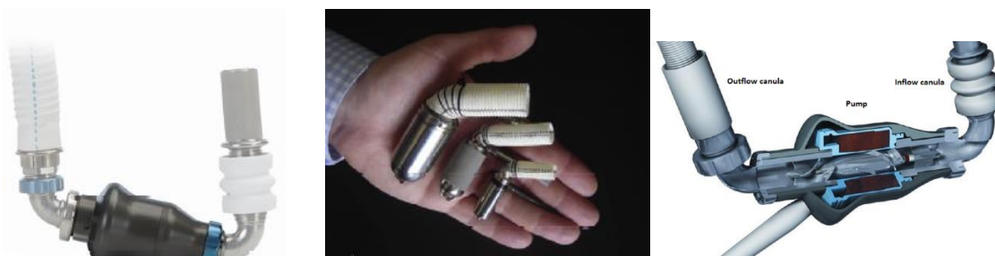
Figure 1.14. Heart Mate II (left) and Jarvik 2000 (centre). Basic pump design (right) consists of a rotor with a cylindrical magnet in it that is subjected to a spinning magnetic field created by motor coils in the housing. The rotor is mechanically suspended and generated momentum in the blood thanks to curved blades mounted on its body.
