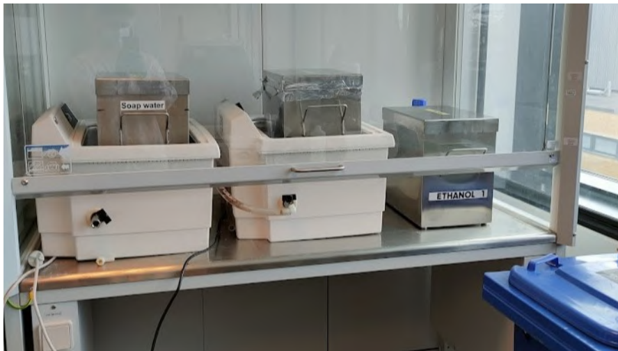
Figure 4.1: The cleaning setup inside DTU Multilab. Three separate bathtubs: hot soap water, deionized water and ethanol.
