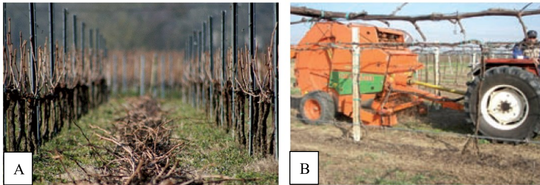
Figure 3.18: A) Rows of vine prunings between the rows. B) Baler in operation during the collection phase
