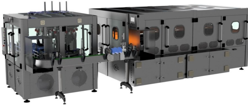
Figure 3.22: Tunnel Heating bottles: Dynamic radiant air conditioner
