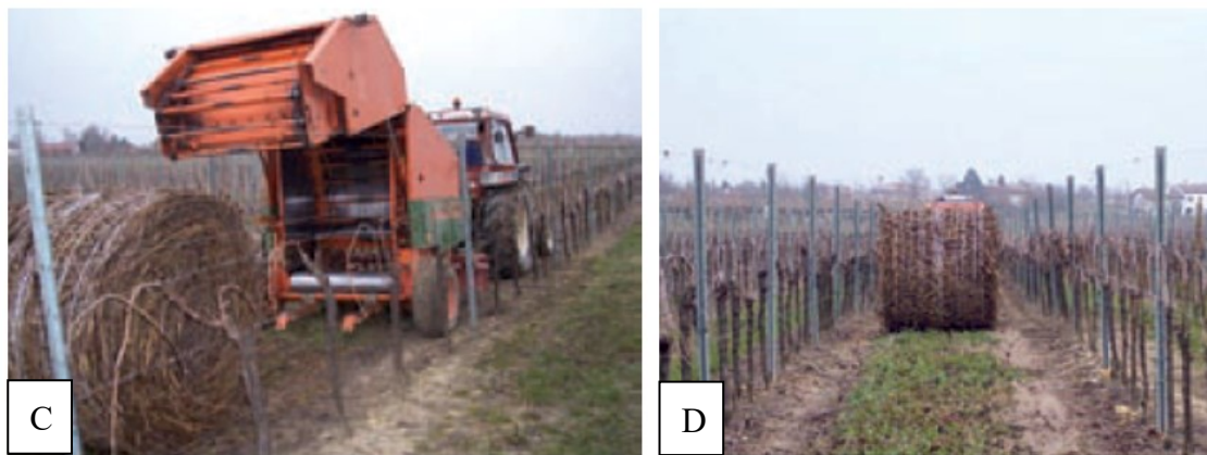
Figure 3.19: C) Baler in operation during the release of the bale wrap. D) Bale wrap of vine prunings.
