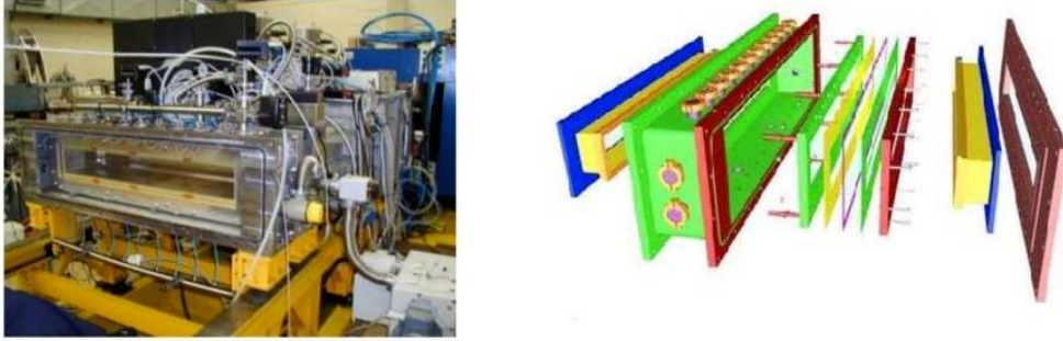
Figure 2.5: Picture (left) and design (right) of the MWPPAC of PRISMA. Taken from [8].
