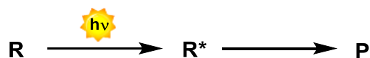
Figure 4. General scheme of direct photochemical reaction. R: reactant; R*: reactant in an excited state; P: product.
