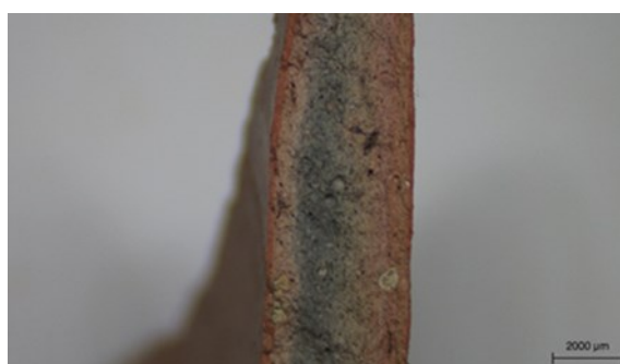
Figure 22 – Photomicrograph of organic remains as observed microscopically (in plain-polarised light) and photo from the stereomicroscope on the fresh cut. From top to bottom: sample 23, 54, 36, 47
