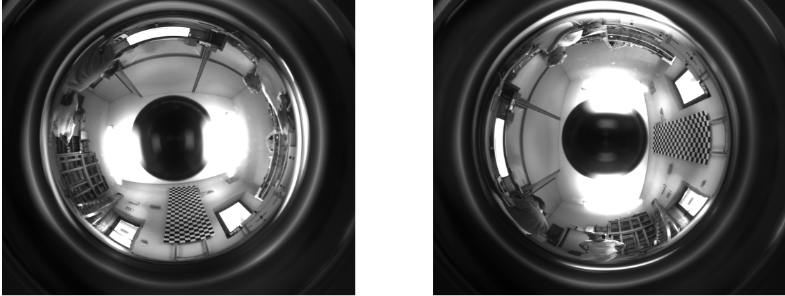
Figure 3.4: Examples of images acquired for the calibration procedure, here with chessboards 28 squares long and 10 squares wide.
