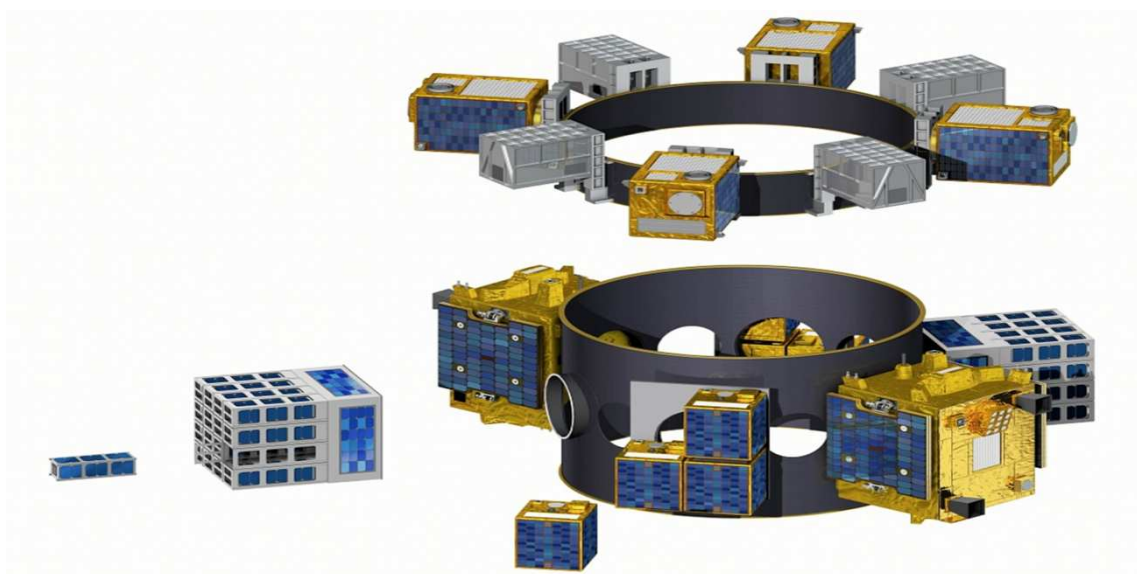
Figure 1-3: Piggyback configuration used by ESA in 2019.
