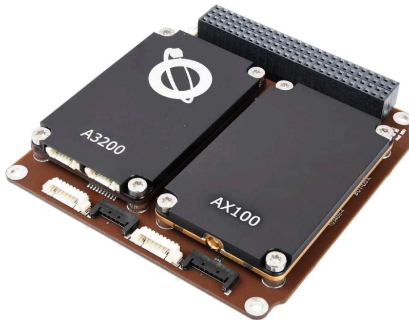
Figure 2-9: Configuration of the NanoDock DCM-3 with NanoMind 3200 and NanoCom AX100 boards.
