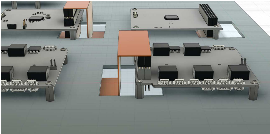
Figure 3-5: Top view of the opening to allow the connection of the boards made with Fusion 360.
