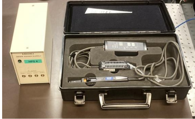
Figure 4.6 Hioki Current Probe based on Hall-effect
