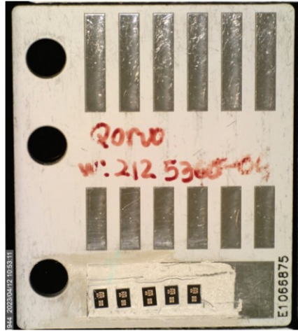
Figure 2.1 Example of a chip under test with 5 GaN HEMT transistor from QORVO on it. The picture has been taken with Dino lite microscope camera.
