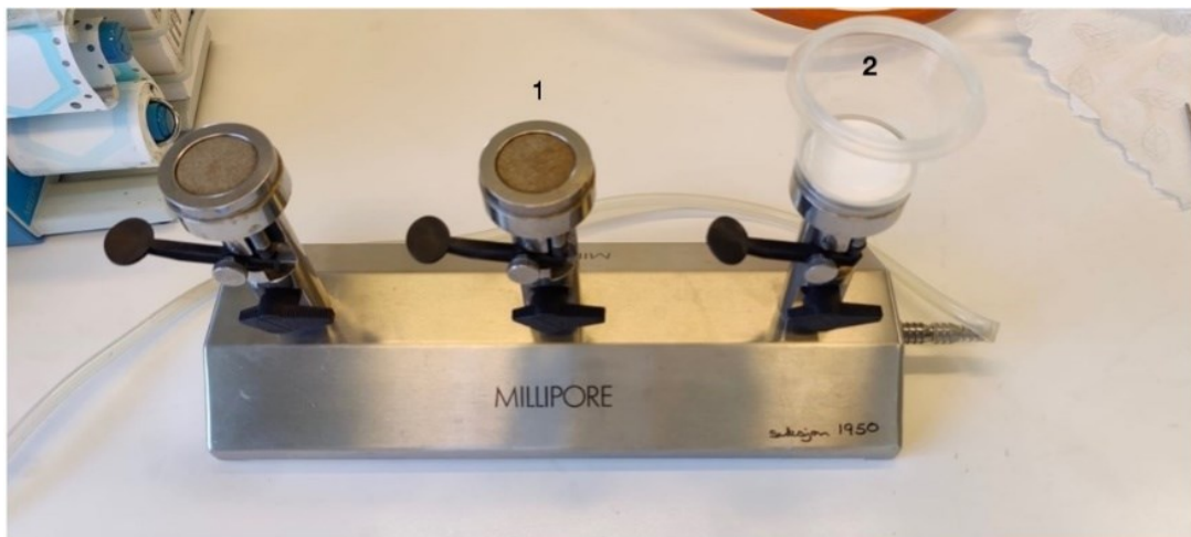
Figure 6: vacuum pump used to filtrate the water samples, before the filter in place (1) and with both filter and fennel in place (2).
