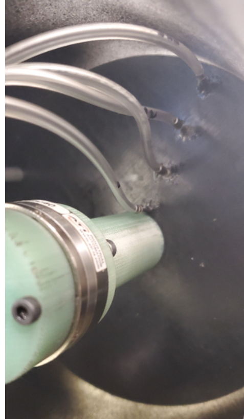
Fig. 14: Internal Model Image of ATI Mini-40 Load Cell and Pressure Taps
