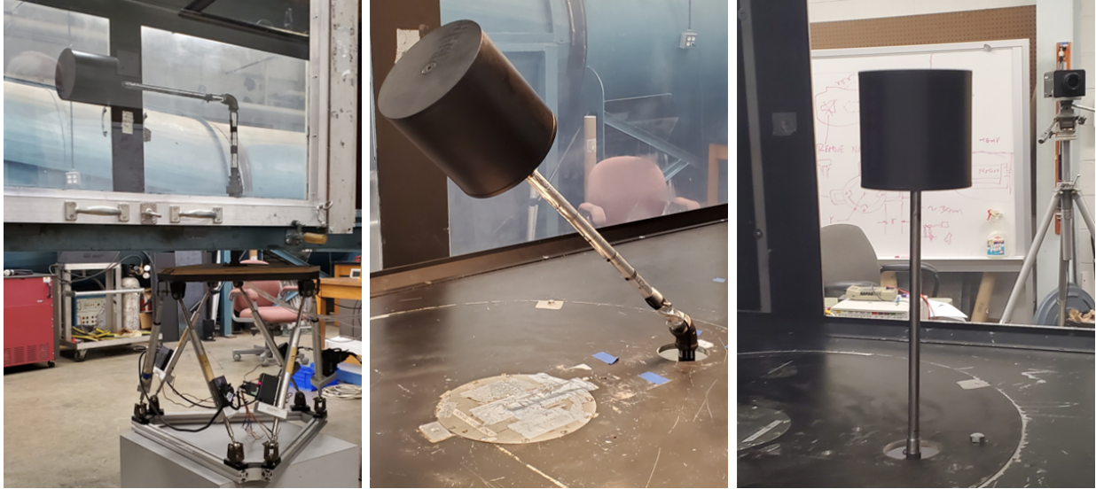
(a) 0° Pitch Angle Fixture with Stewart Platform (b) 45° Pitch Angle Fixture (c) 90° Pitch Angle Fixture
