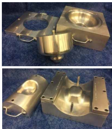
Figure 5: Forming dies for end caps (top) and pole (bottom).
