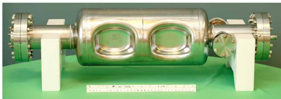
Figure 11: Final welded 2-cell rf-dipole cavity.
