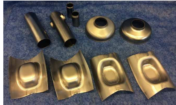
Figure 6: Formed poles, end caps and beam tubes.
