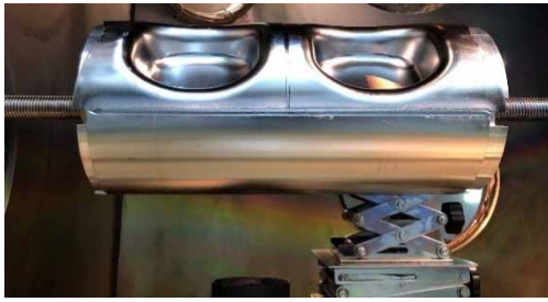
Figure 9: Center body welding in the EBW machine.
