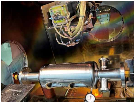
Figure 10: Final welding of the 2-cell rf-dipole cavity.
